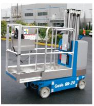
Sliding Mid Rail Extension Deck Platform 55 x 29.5 in (140 x 75 cm) provides 20 in (51 cm) of horizontal outreach and a larger work area within the platform.
